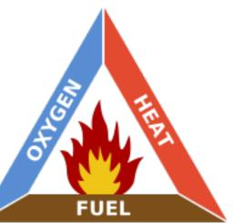
the water to remove the heat from the triangle, whereas a CO2 extinguisher removes the oxygen. A foam extinguisher aims to remove both, with the foam acting as a cooling agent but also a barrier to prevent further oxygen from reaching the fuel source.
