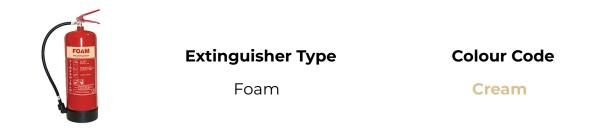
Foam extinguishers are suitable for use on both Class A and B fires which makes them a good option for many environments. The foam acts as a rapid coolant and prevents oxygen from reaching the fire. Foam extinguishers have a cream panel. Foam extinguishers work by smothering the fire and cools via the water content which helps to prevent it from reigniting.
